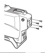
Attach the battery adaptor mounting bracket (Part number 3-690-850-01; not supplied) with the screws removed in step 1.
